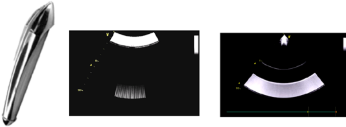
Figure 3 The „Nickel tool“ and the test result images. The image on the left shows the response from a convex transducer where width of aperture and number of elements is observable. The right image was obtained by use of a phased array sector transducer. The centre frequency of this transducer is low (cca 2 - 3 MHz) therefore the third deep strip only is visible and the whole lateral area is marked because in the phased array system the signal received by one tested element is distributed to all receiving channels. (From Sonora leaflet.)
